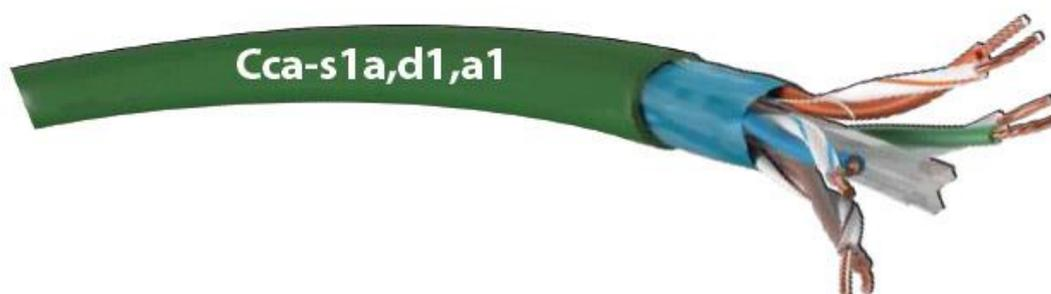
**CODICE      DESCRIZIONE****205.0075.70** Cavo FTP Cat. 6 guaina LSOH 4X2X24 AWG in bobina da mt. 300/500
